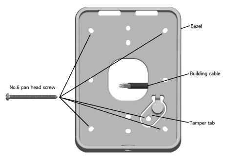
5. Connect the reader tail extending from the facia assembly to the building cable. Connect the wires for the HBUS device to interface.
