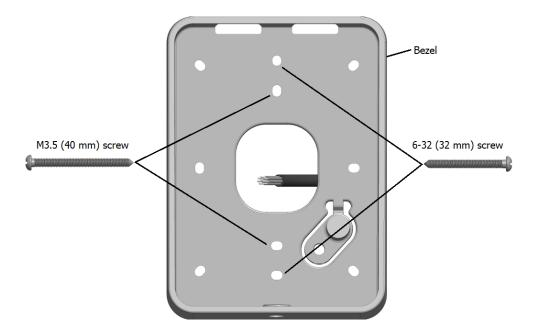
4. Drill pilot holes for the four corner fixing holes and the tamper tab. Secure the bezel to the mounting surface using the four corner fixing screws provided. Secure the tamper tab (located in the bezel) to the mounting surface using the remaining fixing screw provided. It is important the four corner fixing screws are used to ensure the reader is flush with and tight against the mounting surface.
