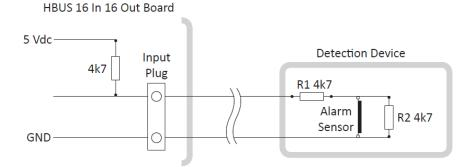
Resistor values can be configured for a HBUS 16 In 16 Out Board in Command Centre (via the EOL Resistors property page). Refer to the topic "Configuring EOL Resistors for devices" in the Command Centre Configuration Client Online Help.
