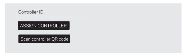
Note: If you're unable to scan the controller's QR code, you can enter the controller's ID in the **Controller ID** field, then click the **ASSIGN CONTROLLER** button. The controller's ID is printed on the controller, below the QR code.
